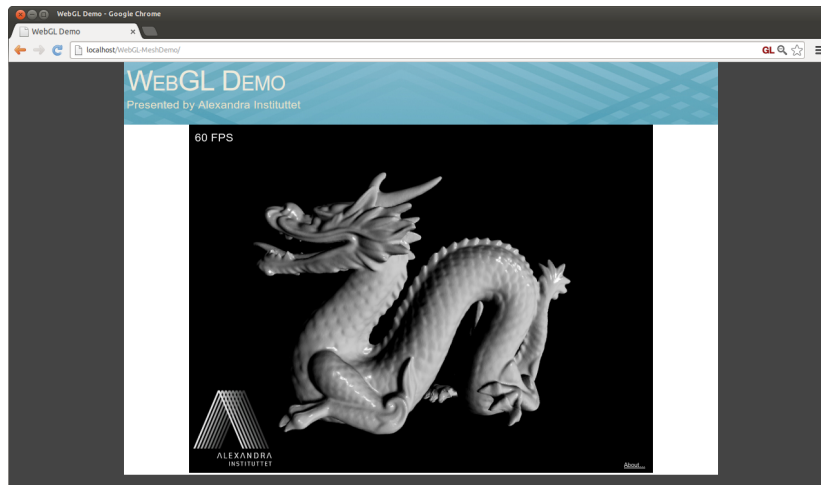
Figure 1: The Stanford dragon consists of 871414 triangles. Models with this polygon count are straightforwardly rendered in real time in WebGL. A big challenge, however, is how to load the massive amounts of vertex data for such detailed models. For example, the model shown in the figure uses 60 megabytes of vertex position and normal data.
